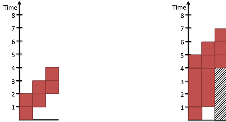
Figure 4.3: Block C is non-rigid and has a unique equilibrium. After stacking it once, the resulting upper contour is different depending on what the initial condition is. However, after stacking the block again, the upper contour is the same because it converged to the same equilibrium value regardless of the initial condition.
