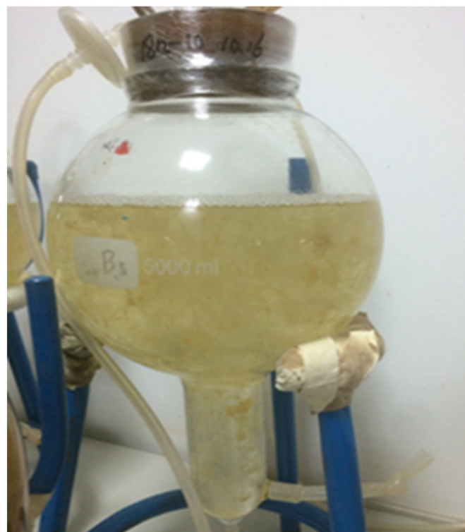
Fig. 1. Adventitious roots of P. ginseng cultured in a 5-L airlift bioreactor for 30 d.
