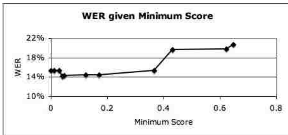
Figure 4.3: WER on the training set for minimum scores required to be included in the output text.
