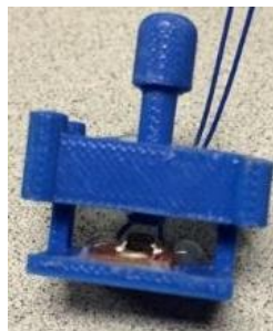
Figure 4.7 IR Photo Reflector with Compliant Mechanism Button
