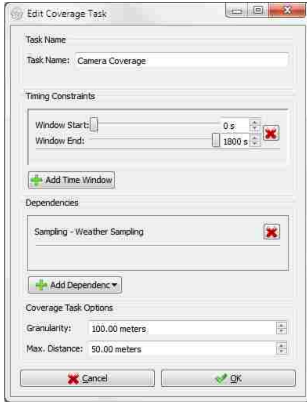
Figure 4.5: A screenshot of the GUI’s coverage task editor. Each task type (coverage, sampling, fly through) has its own specific options as well as some (timing constraints and dependencies) that are common to all tasks.
