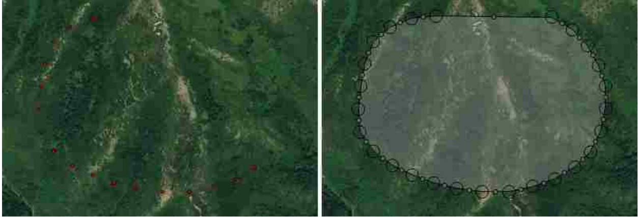
Figure 7.5: An illustration of drawing a circular task area using the improved polygon drawing functionality. The left side of the figure shows the circular area as it is being drawn. Small red dots mark the path the mouse has taken during the drawing. When the mouse is released, the task area is completed, as shown on the right.
