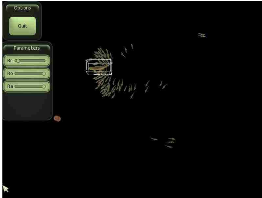
Figure 1.5: A user-controlled agent, marked with a white box, splits the swarm into two groups by repelling swarm members close to it.
