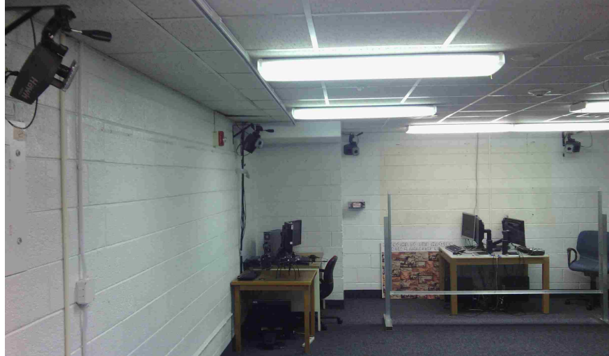
Figure 2.4: The MAGICC lab's motion capture room. The room is equipped with a camera system from Motion Analysis which provides 6DoF tracking with sub-millimeter and sub-degree accuracy at rates up to 200 Hz.
