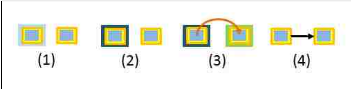
Figure 37: Creating a link. (1) A user’s finger presses an item. (2) After a specified waiting period, the item highlight turns green indicating that a long-press has started. (3) The user drags the item to another item until the other item receives a green background highlight. (4) The user releases their finger and selects “Create Link”. A link is created.
