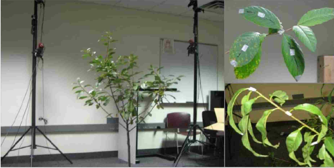
Figure 2.1: Motion capture setup for a natural tree using an optical motion capture system.
