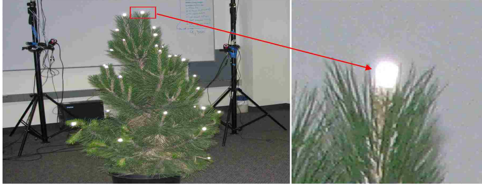
Figure 4.3: Marker placement on the crown periphery avoids occlusion while generating data that can be used to generate crown structure.
