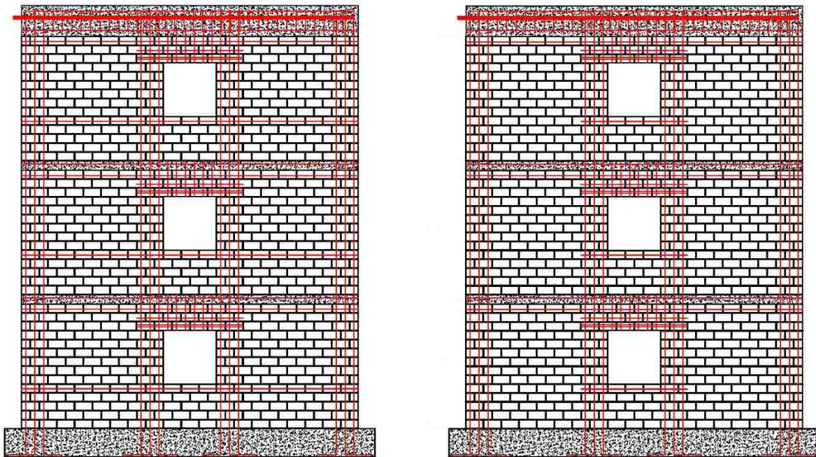
Figure 1-1: Difference in experimental specimens – wall 1 (left) and walls 2&3 (right)
