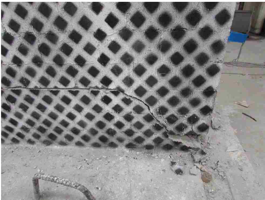
Figure 4-14: Toe crushing of experimental masonry wall
