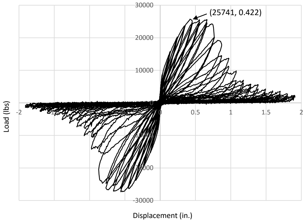
Figure B-32: Hysteresis curve for #4 vertical reinforcement
