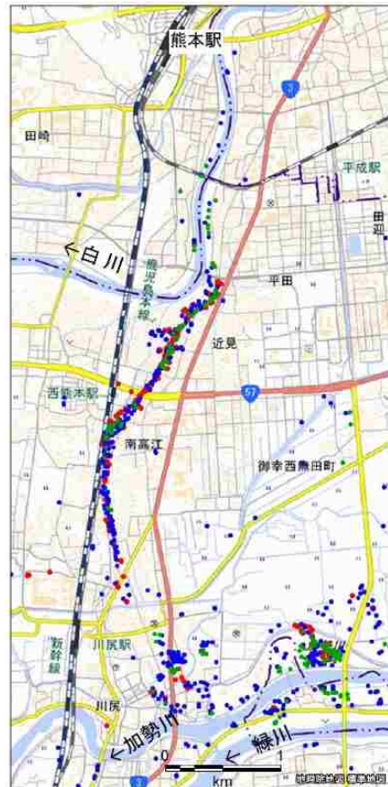
Figure 5-9: N-S liquefied river channel with liquefied sites (Wakamatsu et al., 2016)
