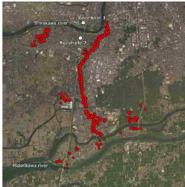
Figure A-7: Observed soil liquefaction in Kumamoto City (Bhattacharya et al., 2018)
