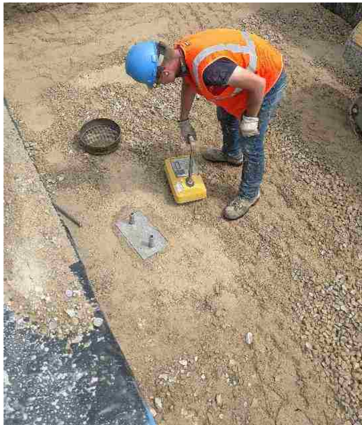
Figure 3-12. The author performing a nuclear density test.
