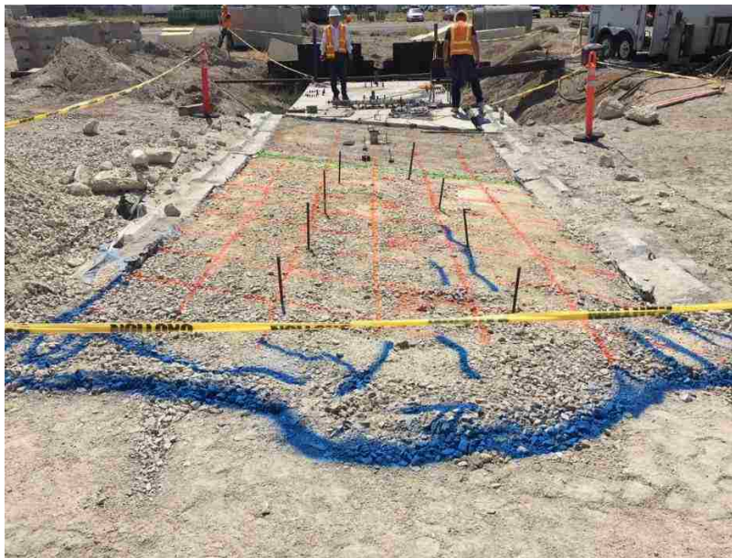
Figure 3-31. 30° skew after passive loading test, showing grid lines in orange and surface cracking highlighted in blue.
