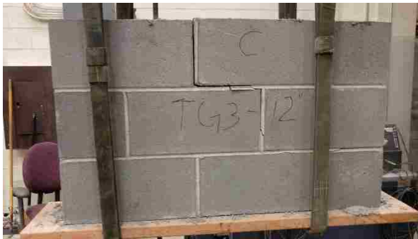
Figure C-13: Test Group 3 Masonry Panel C at Failure
