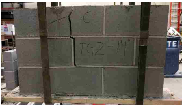
Figure C-10: Test Group 2 Masonry Panels A & B at Failure
