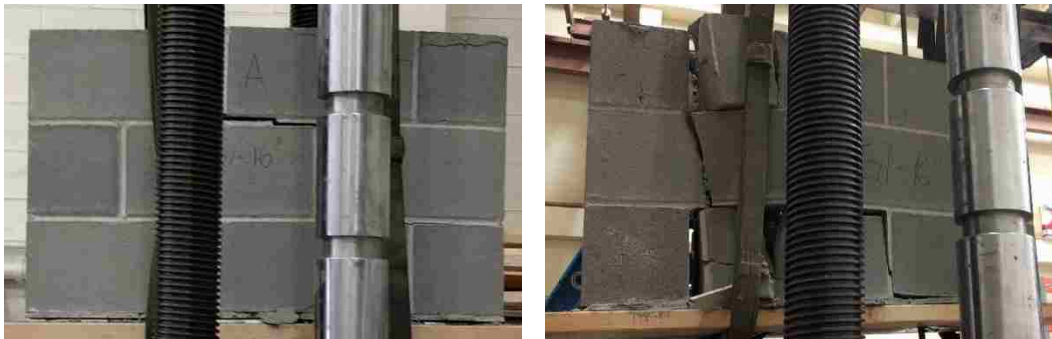
Figure C-6: Masonry Prisms at 28-Day Failure
