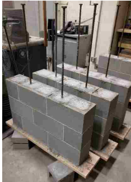
Figure 3-9: Grouted Panels Before Testing
