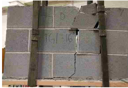
Figure C-7: Test Group 1 Masonry Panels A & B at Failure
