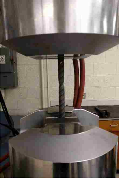
Figure 3-10: Rebar Testing Apparatus
