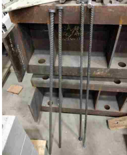
Figure 3-2: Headed Steel Reinforcement
