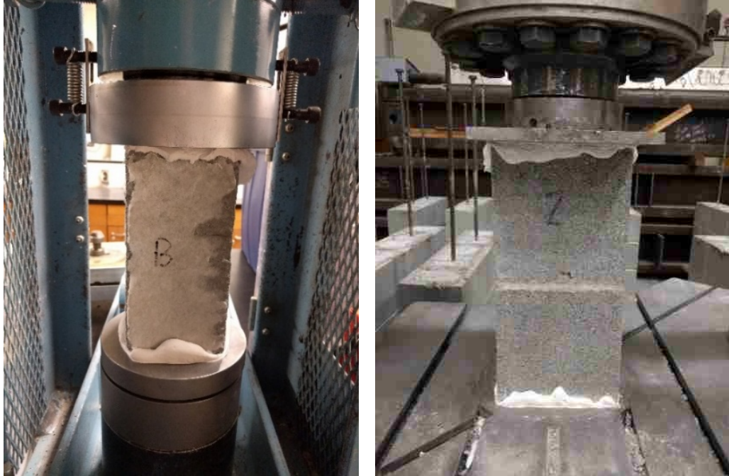
Figure 3-14: Grout and Masonry Prism Testing Apparatus
