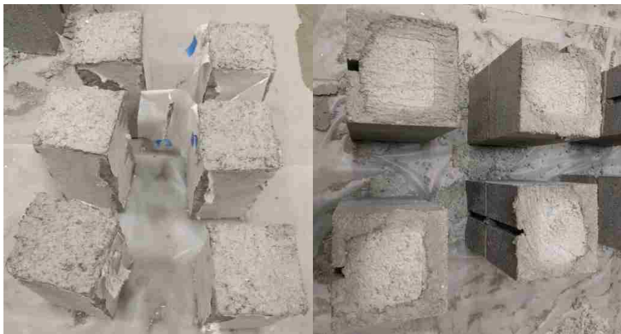
Figure 3-8: Masonry and Grout Prisms
