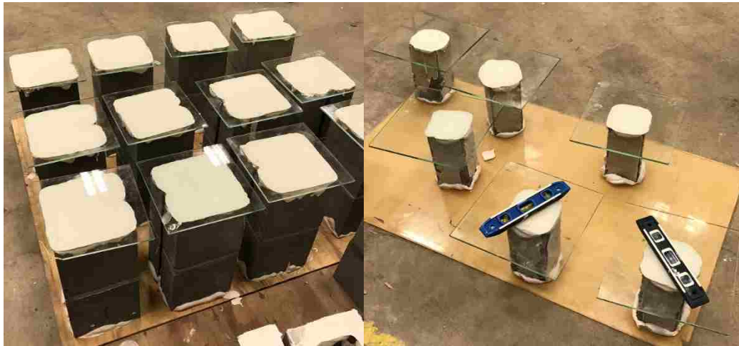
Figure 3-13: Masonry and Grout Prism Capping
