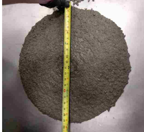
Figure 3-7: Slump Flow Test
