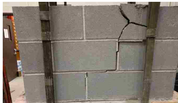
Figure C-10: Test Group 2 Masonry Panels A & B at Failure
