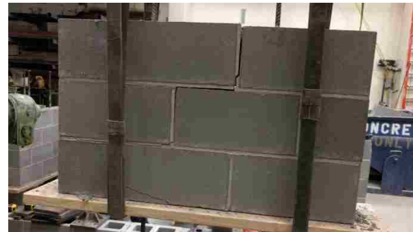
Figure C-13: Test Group 3 Masonry Panel C at Failure
