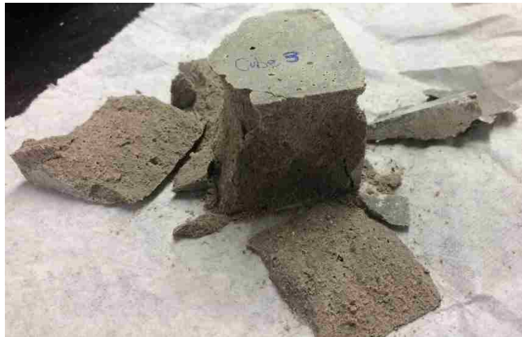
Figure 3-12: Mortar Cube After Compression Testing
