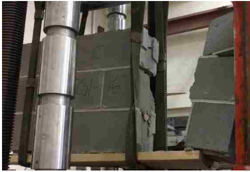
Figure C-7: Test Group 1 Masonry Panels A & B at Failure
