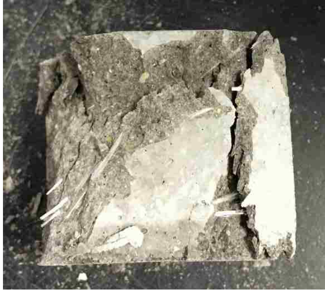
Figure 3-8 Typical failure of surface bond cubes.
