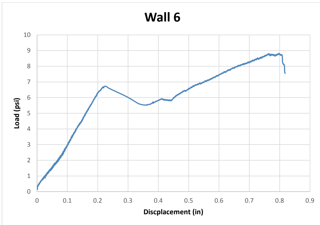
Figure A-15 Load-displacement curve for wall 6.
