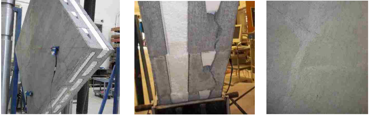
(a) Wallette at failure. (b) Crack of outside webs. (c) Crack down center of wallette.
