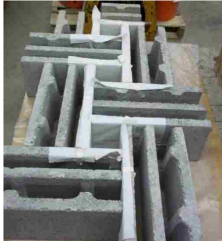
Figure 3-3 Grout prism apparatus.
