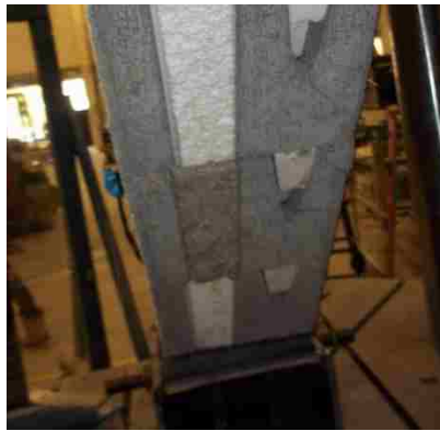
(b) Cracks in web after testing.
