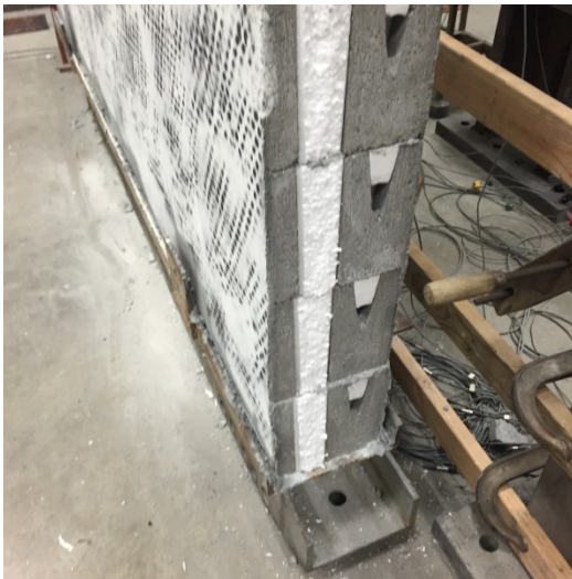
(a) No cracking in webs.
