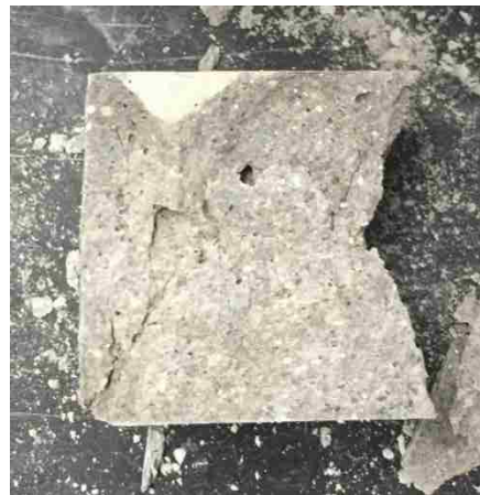
Figure 3-7 Typical failure of mortar cube.
