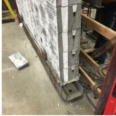
(b) Cracks in webs.
