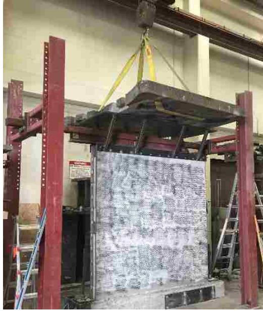
Figure 4-32 Crane counterweight on top of platform above testing frame.
