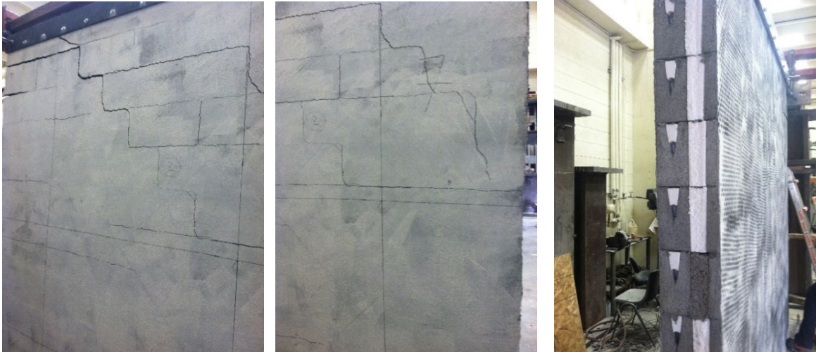
(a) Opening in top course. (b) Typical diagonal cracks. (c) Lack of cracks in webs.
