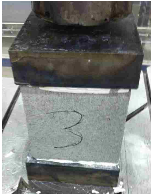
Figure 3-10 Block specimen being tested.
