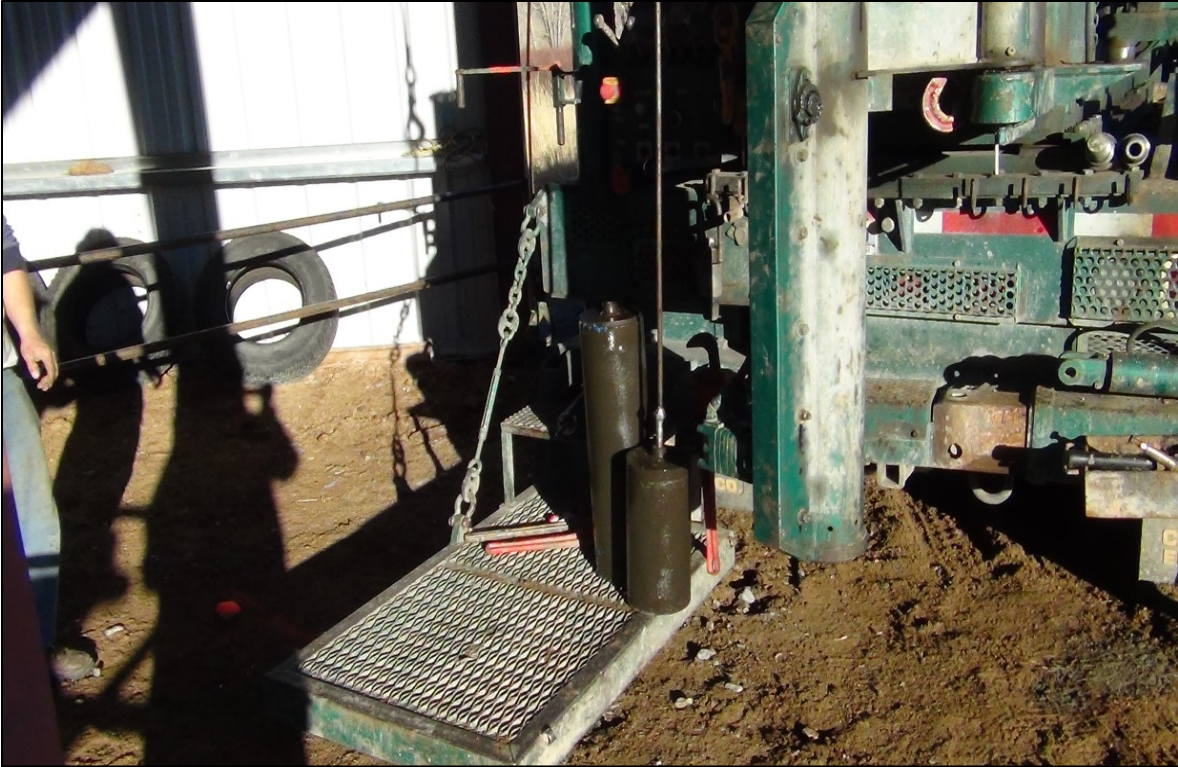
Figure 5-7. View of the two different hammers, the heavy hammer is on the left, 154.4 kg (340 lb.), and the light hammer on the right, 63.6 kg (140 lb.).
