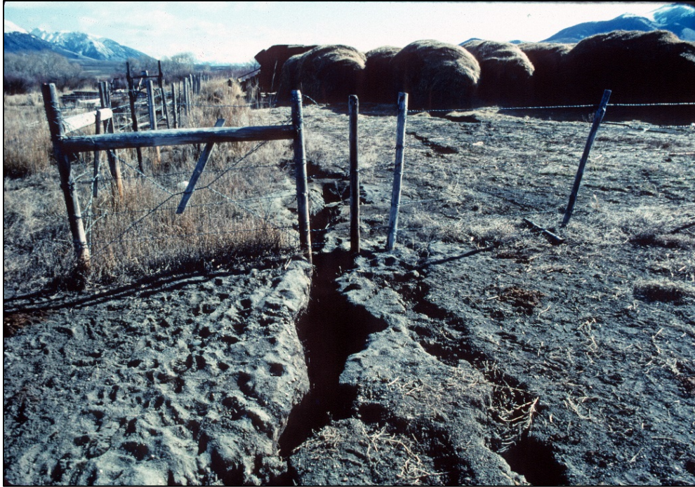
Figure 5-3. Hay yard fence at Pence Ranch, looking south, pulled apart 0.25 m (30 in.) by lateral spread movement (to the left) in 1983. Sand boils erupted along the large fissure leaving deposits on the ground surface (Youd et al. 1985).
