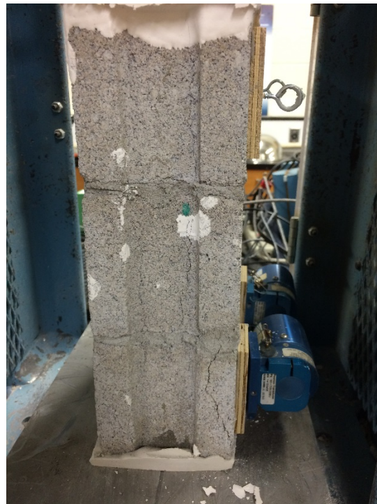
Figure B-5: Testing of CMU Prism using String Pots
