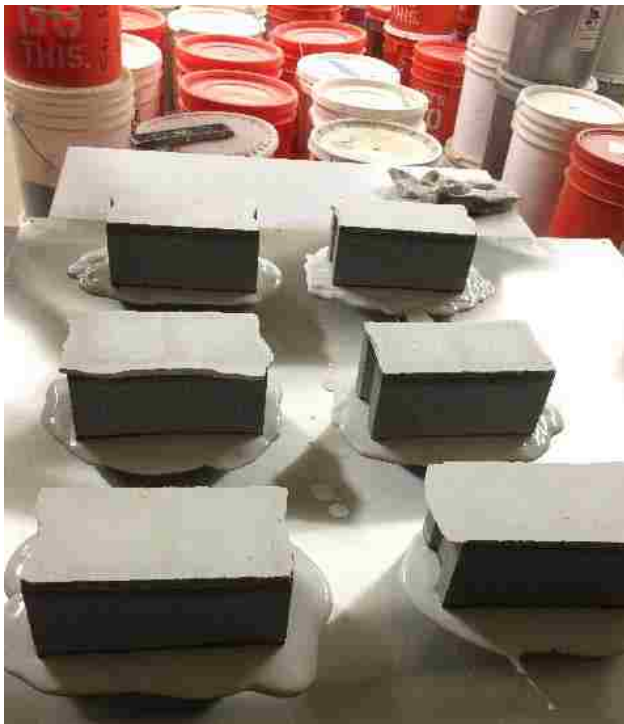
Figure B-1: Capping CMU Blocks
