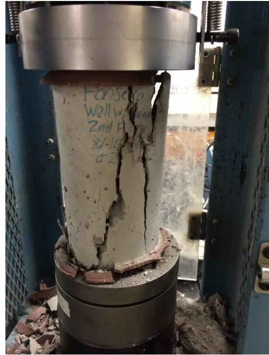
Figure B-4: Testing of Concrete Cylinder
