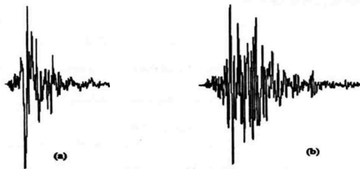
Figure 2-1: Two time histories for earthquakes with similar amplitudes but different frequencies and durations.
