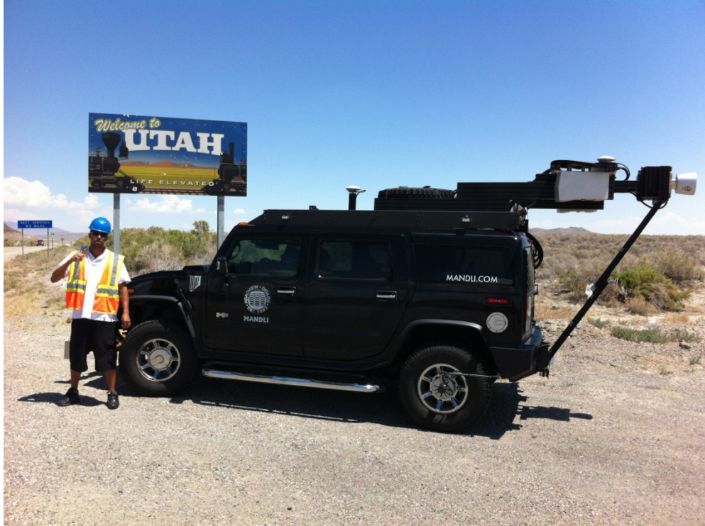
Figure 2-8: Mobile LiDAR vehicle (FHWA 2014).
