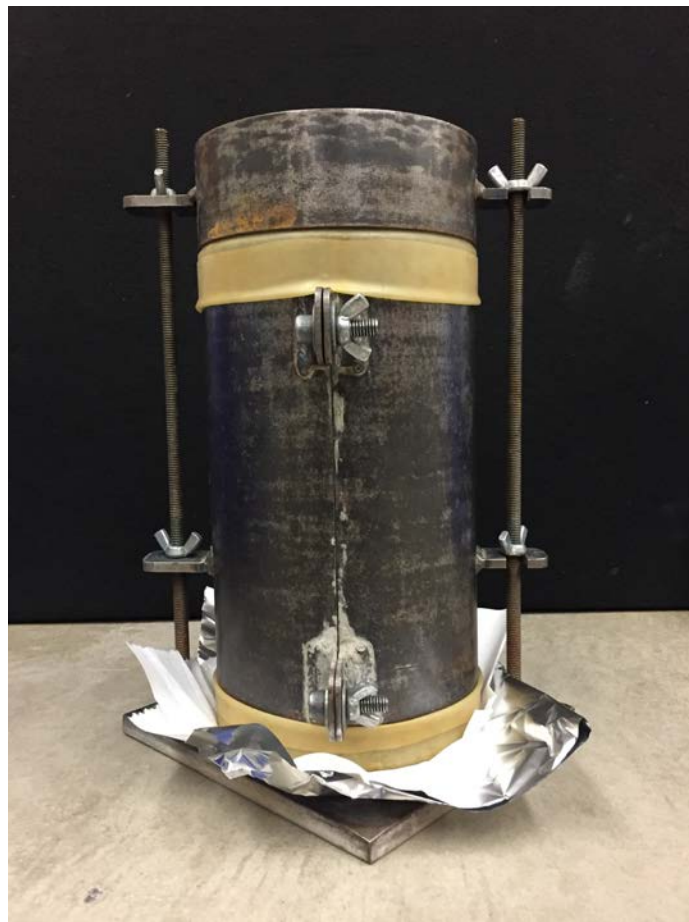
Figure 3-7: Steel split mold for compacting specimens.
