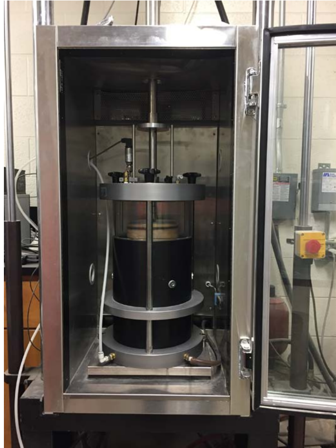
Figure 3-9: Triaxial cell placed inside the UTM-100.
