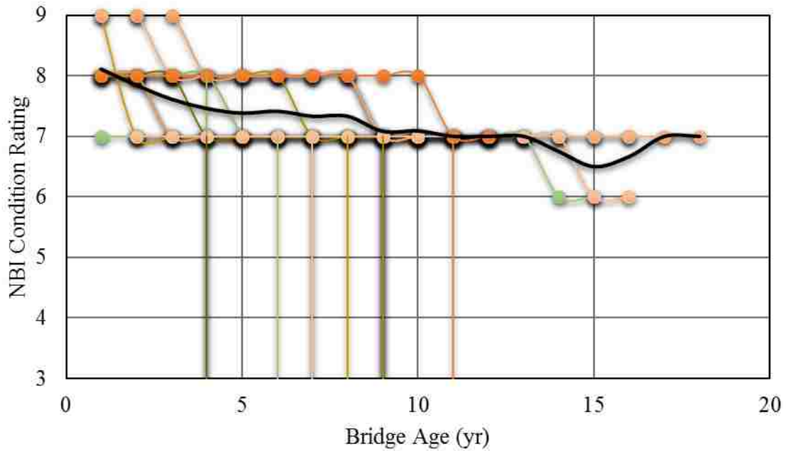
Figure B-4: Individual deterioration curves and average curve aligned by deck construction time for bridge decks with early application of an epoxy overlay in Region 1.
