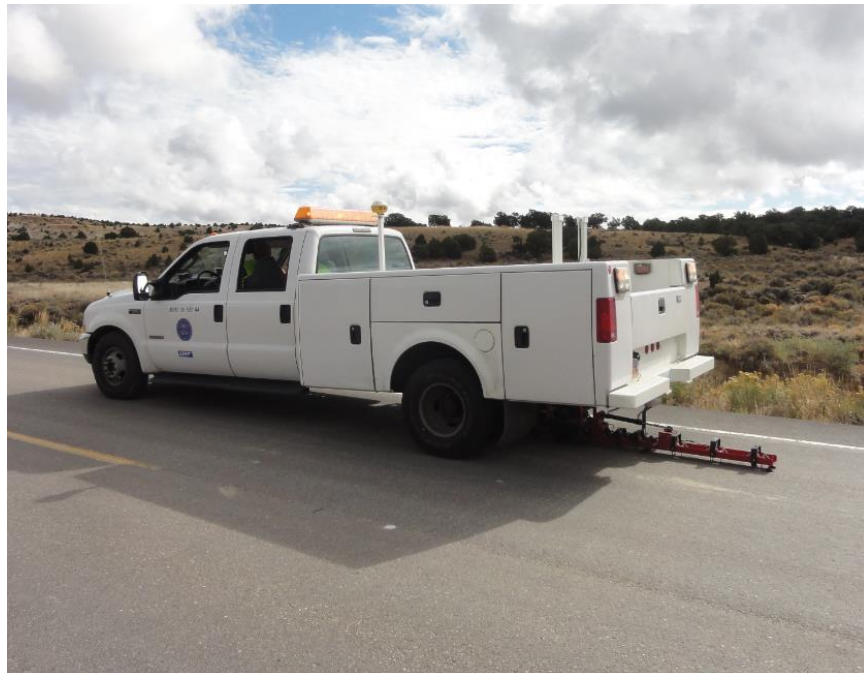
Figure 3-2: FWD testing of pavement structure.
