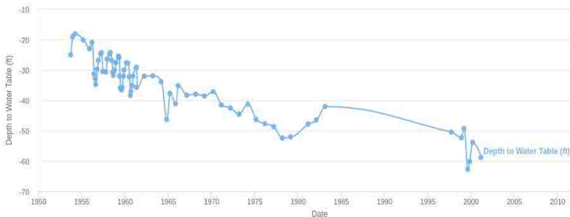
Figure 2-8: Example PCHIP Interpolation
