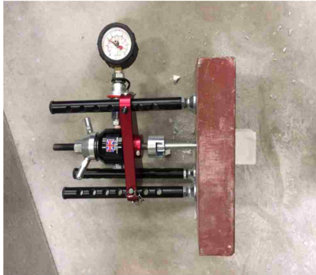
Figure 3-11: Helix Cube Test Setup
