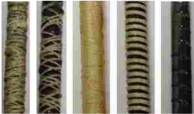
Figure 2.2 Sleeve Configurations (left to right): Full Spiral, Half Spiral, Shrink Tape, Full Braid and Half Braid
