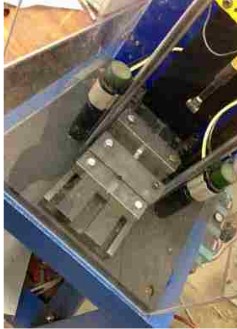
Figure 2.5: Dynatup(R) 8200 Drop Weight Impact Test Machine
