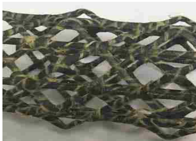
Figure 1.1 Example of a Typical IsoTruss Structure
