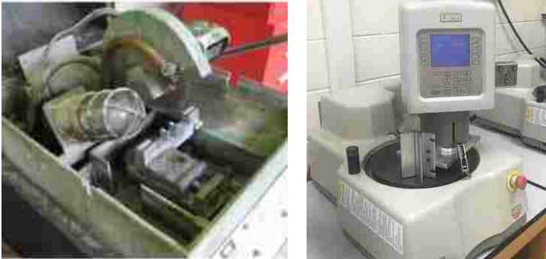
Figure 2.4 Specimen Preparation Equipment: Cutting Jig with Diamond Tip Blade (left); and, Polisher with Vertical Aligning Attachment (right).
