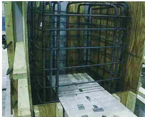
Figure 2.19: Embedment Detail (Harries & Petrou)
