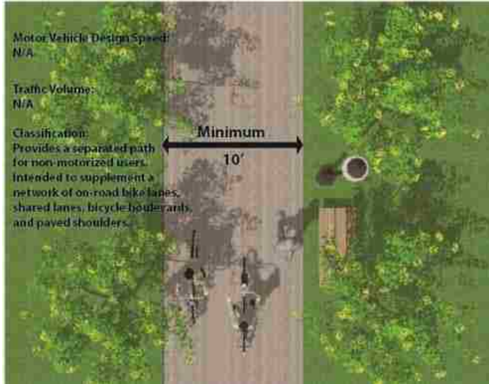
Figure 2-7: Shared use path (independent right-of-way) (MMMPO 2015).
