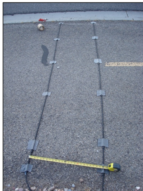
Figure 4-3: Separation of first and second mini tube (photo taken by Chris Haskell, 2015).
