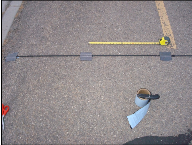
Figure 4-2: Placement of the first mini tube (photo taken by Chris Haskell, 2015).
