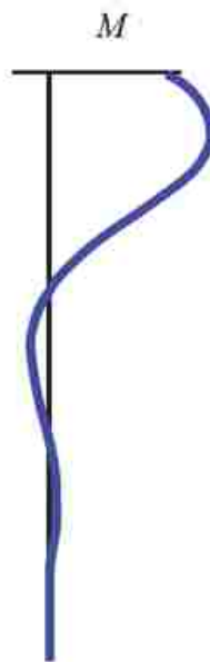
Figure 5-13 Idealized Bending Moment Diagram for a Laterally Loaded Pile
