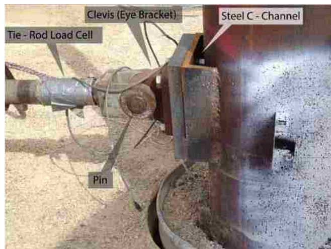
Figure 4-2: Pin Connection
