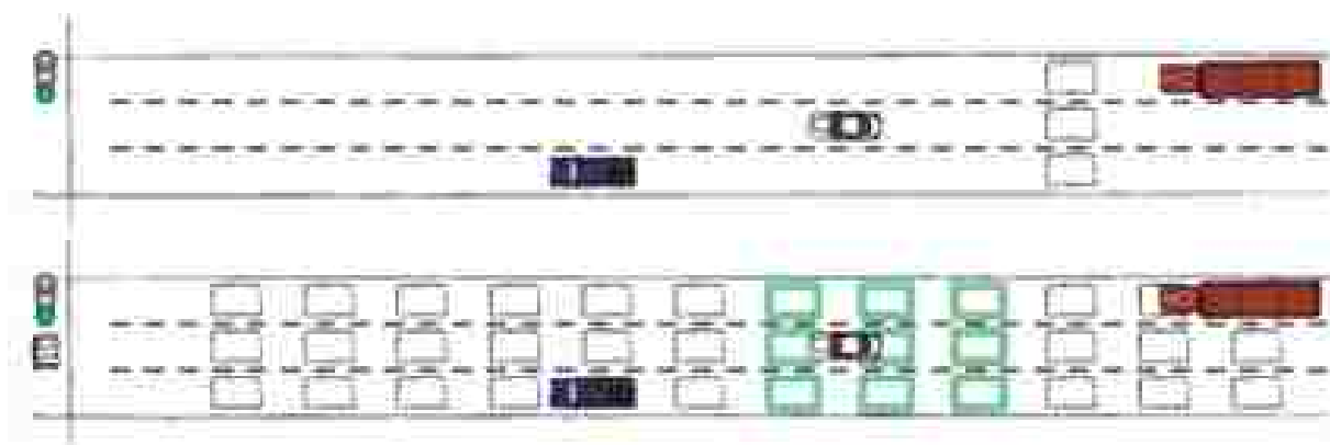
Figure 2-1: Virtual loops created by the sensor for vehicle tracking (Wavetronix 2015a).
