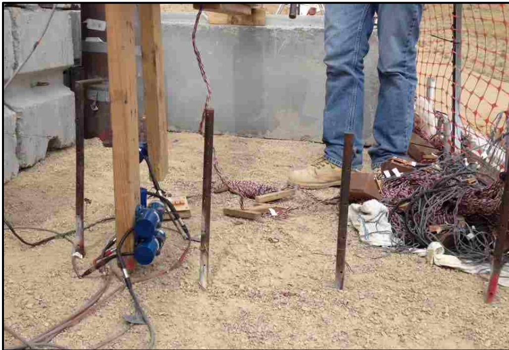
Figure 4-2: Horizontal ground displacement setup.
