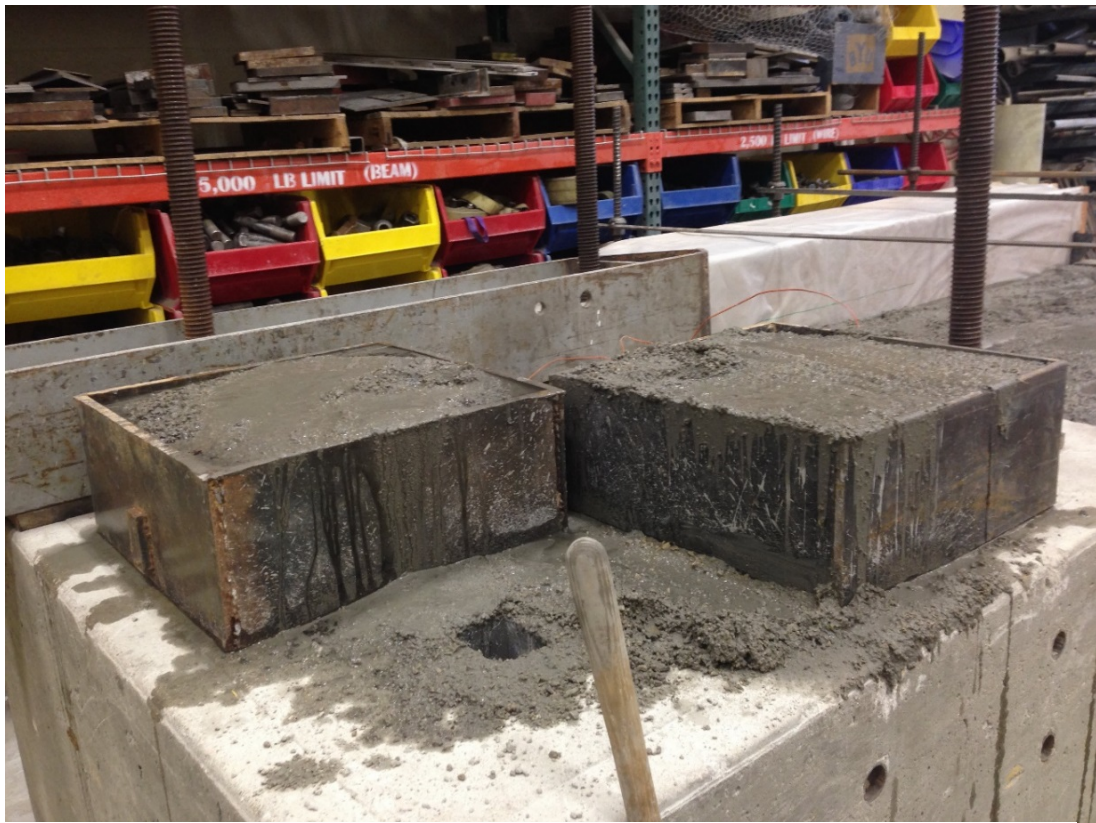
Figure 3-17. Interface shear boxes being filled with CLSM.
