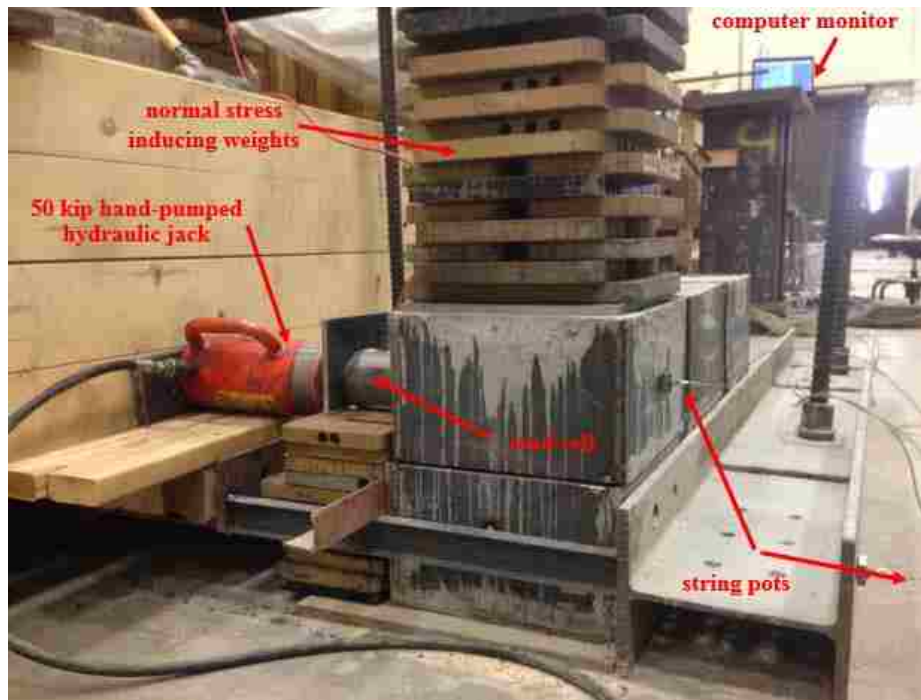
Figure 3-13. Direct shear test set-up.
