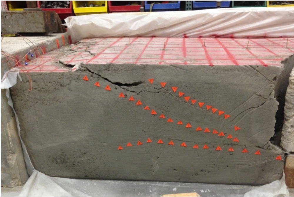
Figure 4-12. Highlighted failure planes.
