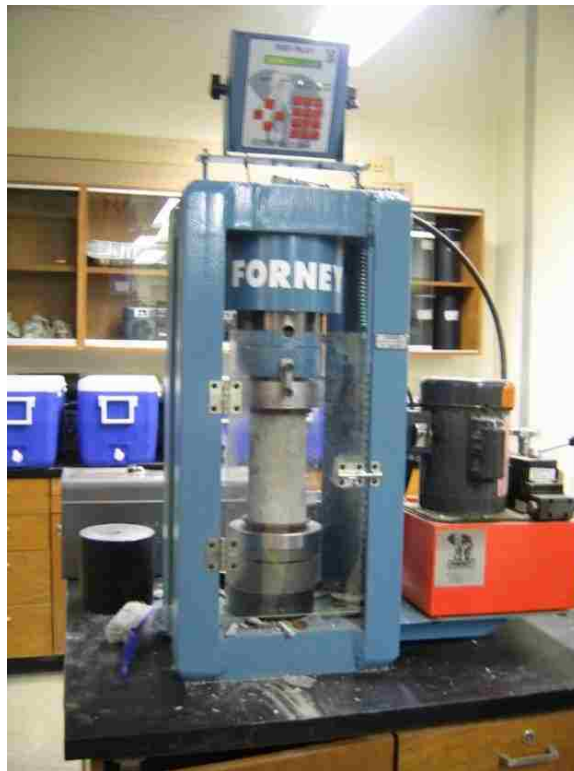
Figure 3-15: Compressive strength testing.
