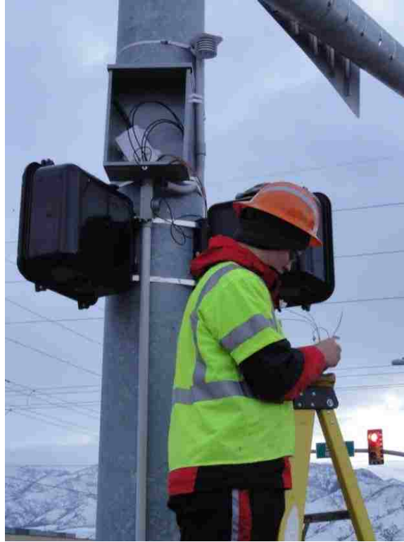
Figure 3-11: Measurement of subsurface temperatures using thermocouple reader.
