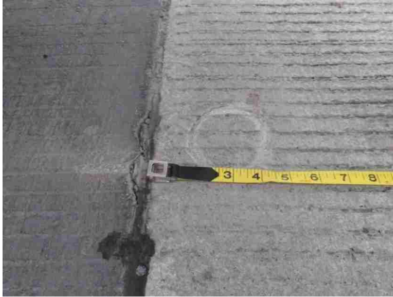
Figure 3-13: Marked beginning point on pavement for roughness survey.
