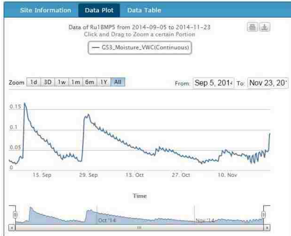
Figure 2-4 HydroServer Site Details Page Showing Soil Moisture at Selected Sensor
