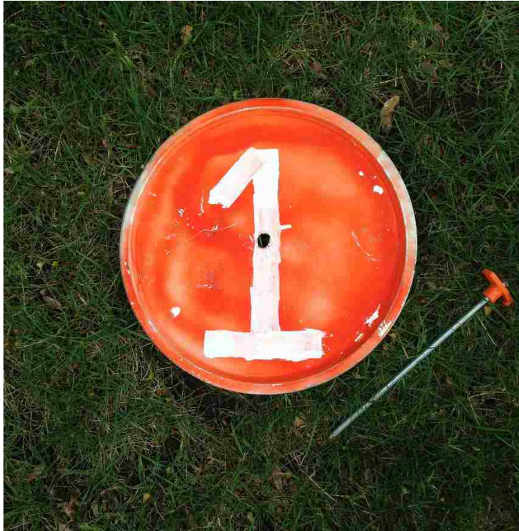
Figure 2-6: GCP Marker Used for This Study
