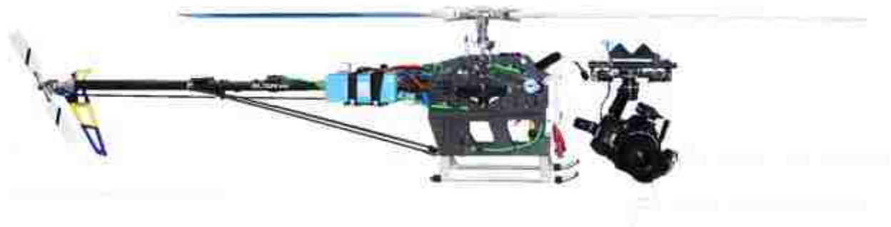
Figure 2-2: Align 800 Helicopter UAV
