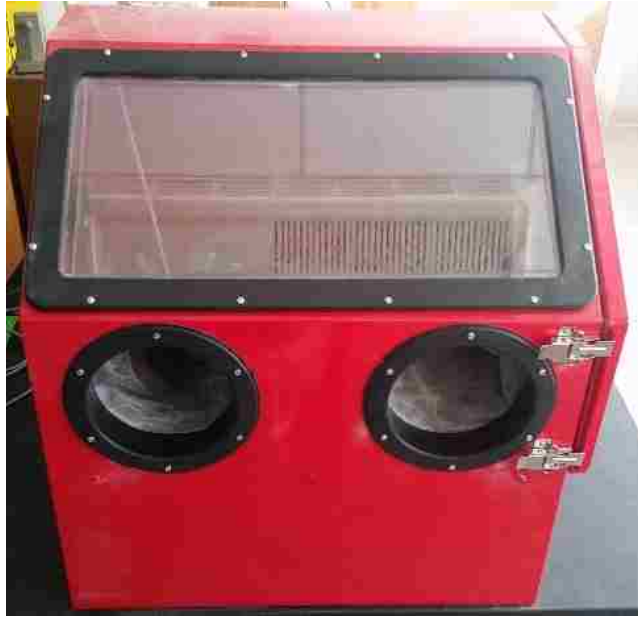
Figure A0-6 Sandblaster used for roughening of glass substrate
