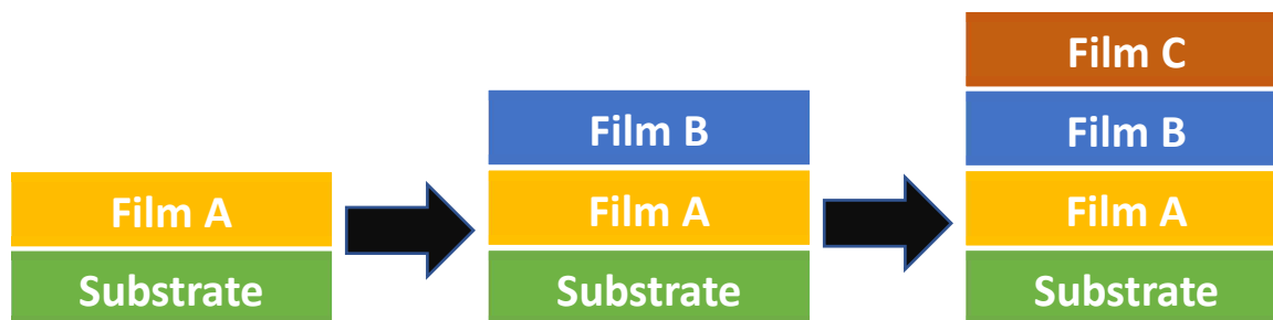
Figure 1-8 General strategy for analyzing multilayer structures, which is to first determine the optical properties of the first layer, then the second layer after its deposition, and so forth. Adapted from Thompkins and Hilfiker Spectroscopic Ellipsometry: Practical Application to Thin Film Characterization 211
