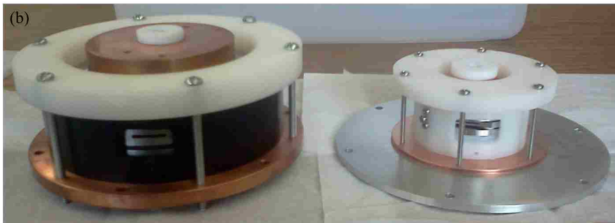
Figure 5-3: Second miniaturized design of the cylindrical toroidal ion trap. (a) Electrode configuration. ( R = 12.05 mm, r_0 = 1.965 mm, z_0 = 1.92 mm) (b) Size comparison of the original cylindrical toroidal ion trap (left) and the miniaturized version (right).
