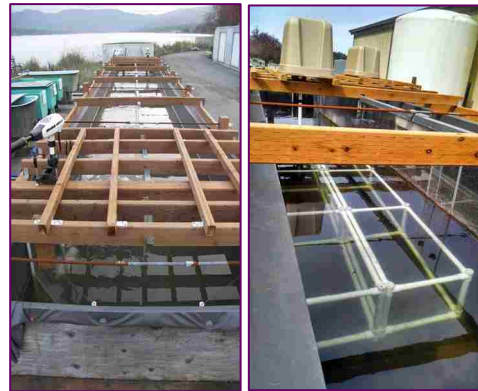
Figure 1.2.2 Top: One of the 500 gal tanks used for the low-velocity studies. Bottom left: Raceway flume used for the high-velocity studies. Bottom right: Frames (empty) used to hold coupons in the raceway.
