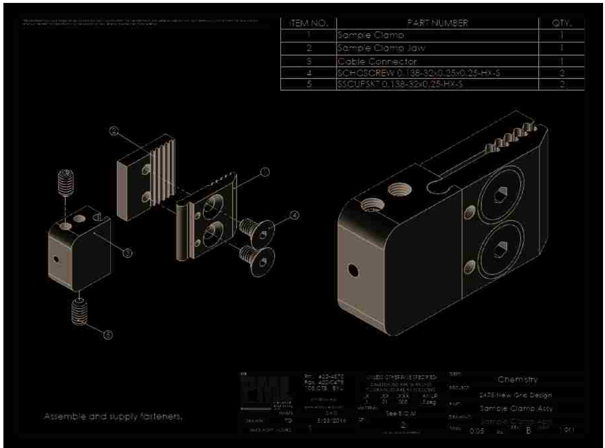
Figure 2.4. Assembly drawing of a sample clamp used with the live pull adapter for current sample mount.
