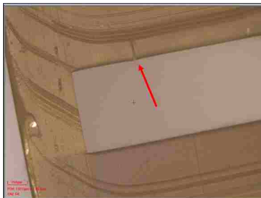
Figure 3.5 Side view of monolith window cracking taken with the profilometer. Red arrow indicates a place where the device is cracked.
