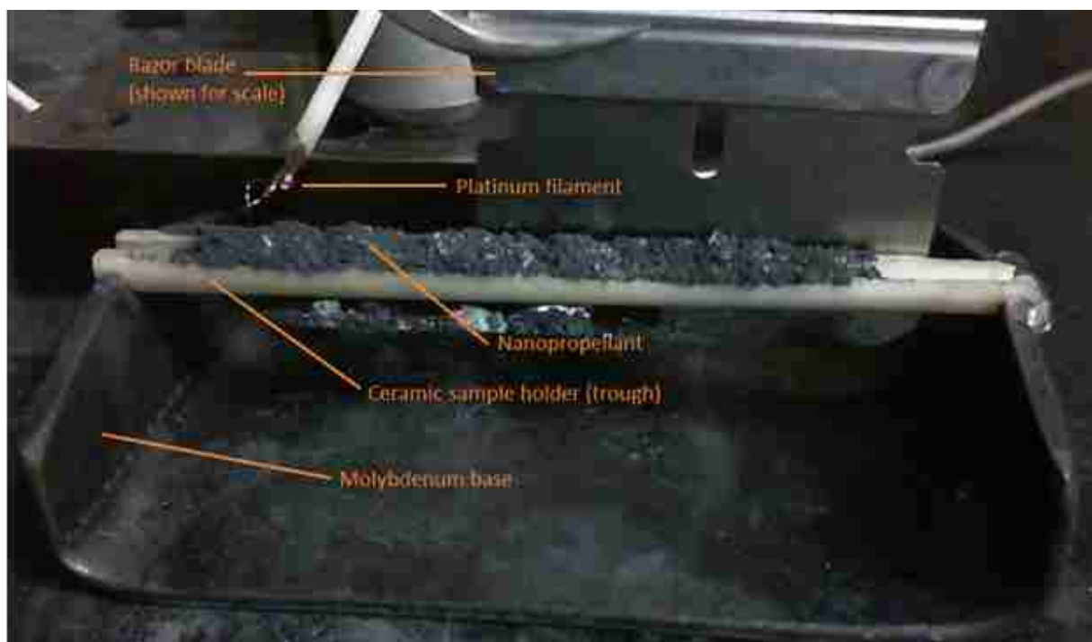
Figure 8 - 1. Test set-up for mass composition ratio optimization burn tests. Shown from the top to bottom are the platinum filament for ignition, a sample of nano propellant, the ceramic sample holder, and the molybdenum base plate. A razor blade was included to illustrate the scale used for this experiment.
