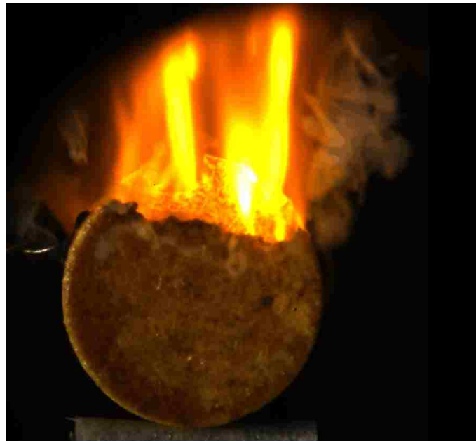
Figure 9 - 2. Image of perchlorate-ferritin pellet burning at 500 PSI. Ferritin is on the front facing portion of the pellet. (Image captured from Video 8-1)
