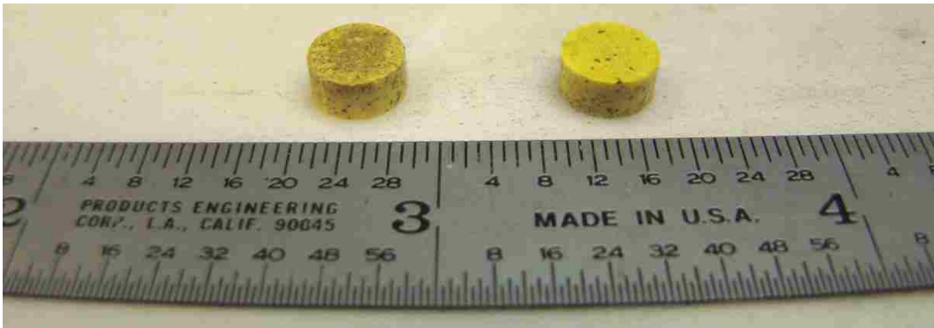
Figure 9 - 1. Pressed perchlorate-ferritin pellets with binder material.
