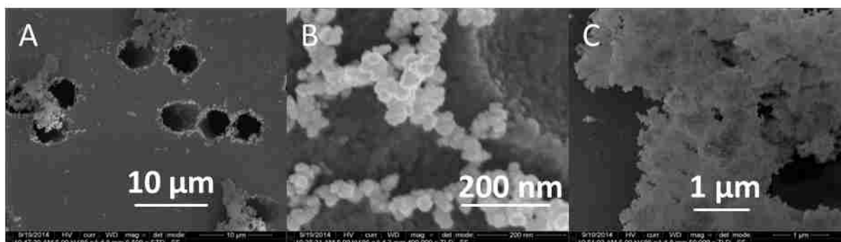
Figure 3.7 SEM images of aerosol particles generated during ablation of scandium aluminum, collected on various pore size polycarbonate filter disks. Scales are listed on each image.
