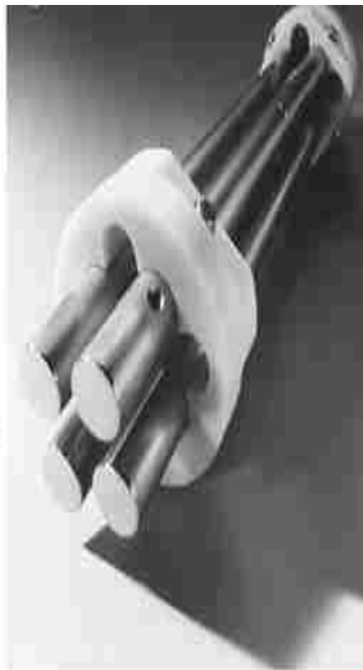
Figure 1.3. Schematic of Linear quadrupole. (Reprinted with permission from Gross, J. Mass Spectrometry, 2nd ed.; Springer, 2011; pp 147)
