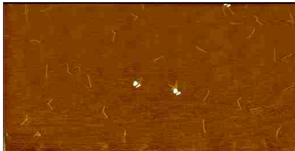
Figure 2.3. AFM image of tight bar origami. Height scale is 10 nm. Image dimensions: 5 \mu\text{m} X 10 \mu\text{m} .
