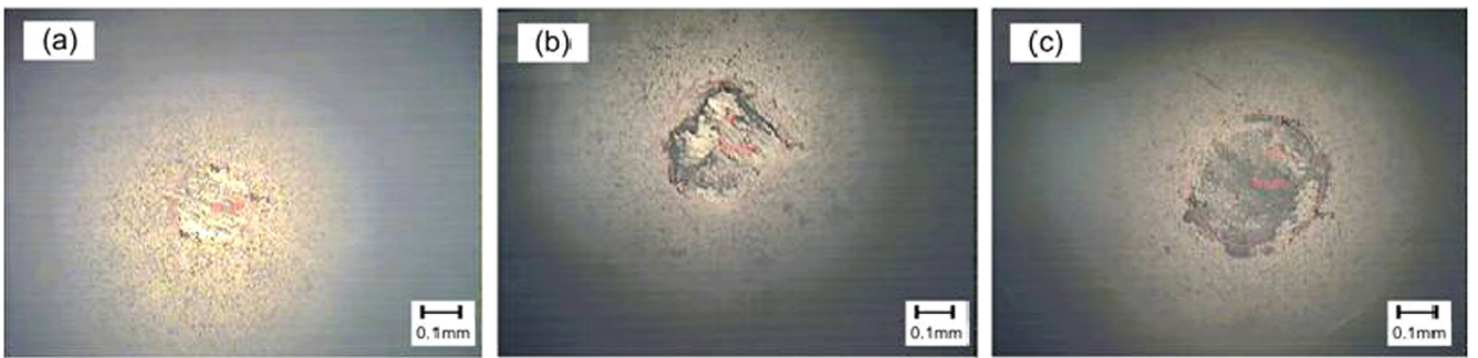
Fig. 12. Wear scar and coating debris on chrome steel ball following Pin-on-disc testing of complex GLC coating in air after a sliding distance of 360 m under an applied load of (a) 20 N, (b) 40 N, (c) 80 N.
