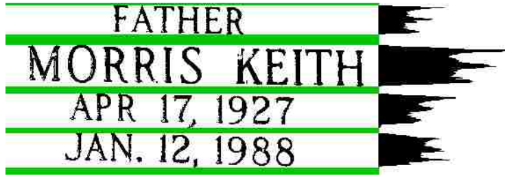
Figure 3.20: A text region where the projection profile is used to create individual text lines. The green regions represent horizontal scan lines where the profile was zero (i.e. no black pixels) and regions that will be discarded.
