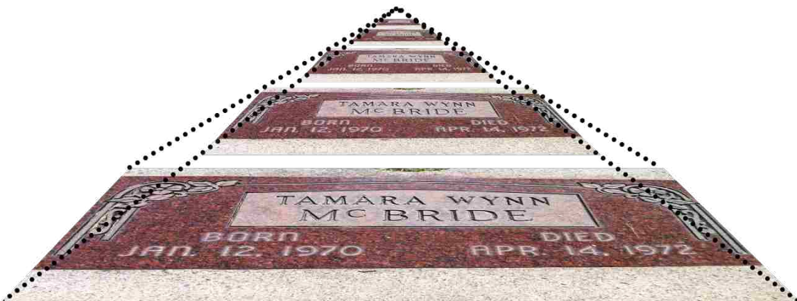
Figure 3.2: A representation of an image pyramid in which each level of the pyramid was created by scaling the previous level by 50 percent. The shown pyramid was created from the image used in Figure 2.5.
