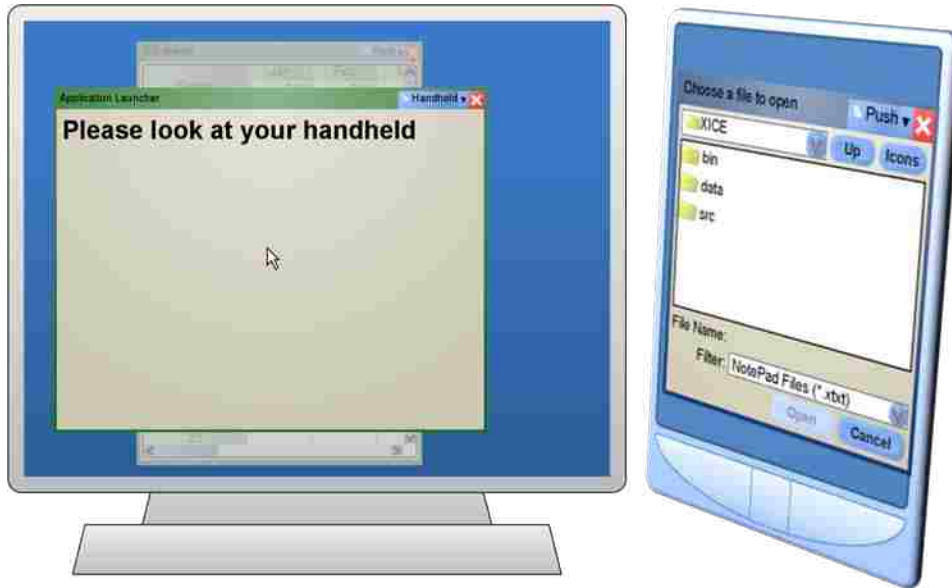
Figure 2:37 – File dialogs are not sent to public displays. Instead, a heads-up dialog rendered on the public screen directs users to the file dialog’s UI on the personal device.
