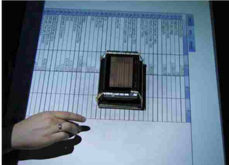
Figure 2:9 – Handheld Spilling: a UI is shown both on a handheld and tabletop computer. The user may interact directly with data through the handheld, and may scroll via the tabletop.
