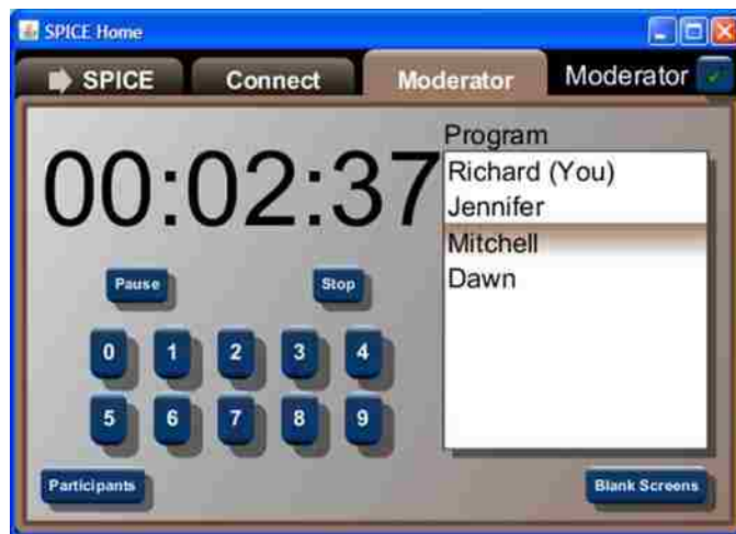
Figure 5:8—Possible moderator software UI. The person selected on the right is the floor. The countdown on the left is used to time the current speaker.
