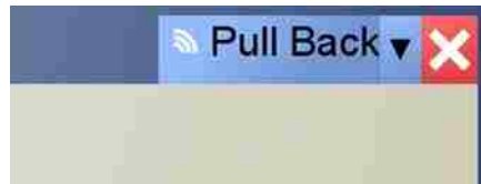
Figure 2:30 – A window’s UI that has been pushed from a personal device to a display server has a "Pull Back" button that enables the user to easily remove that window’s UI.
