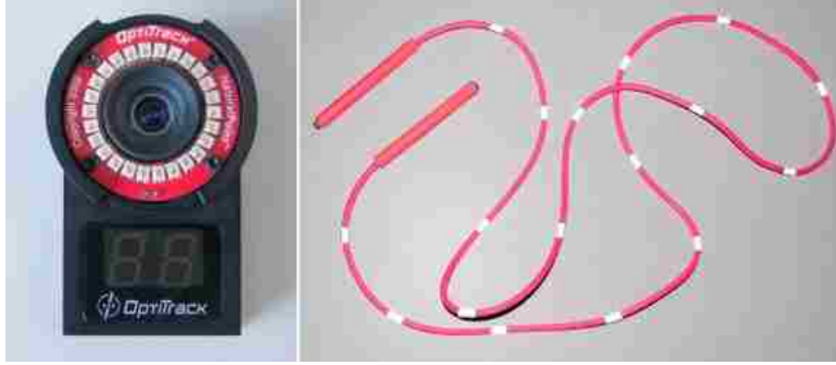
Figure 3.2: OptiTrack Flex camera(left), jump rope wrapped with reflective tape(right)
