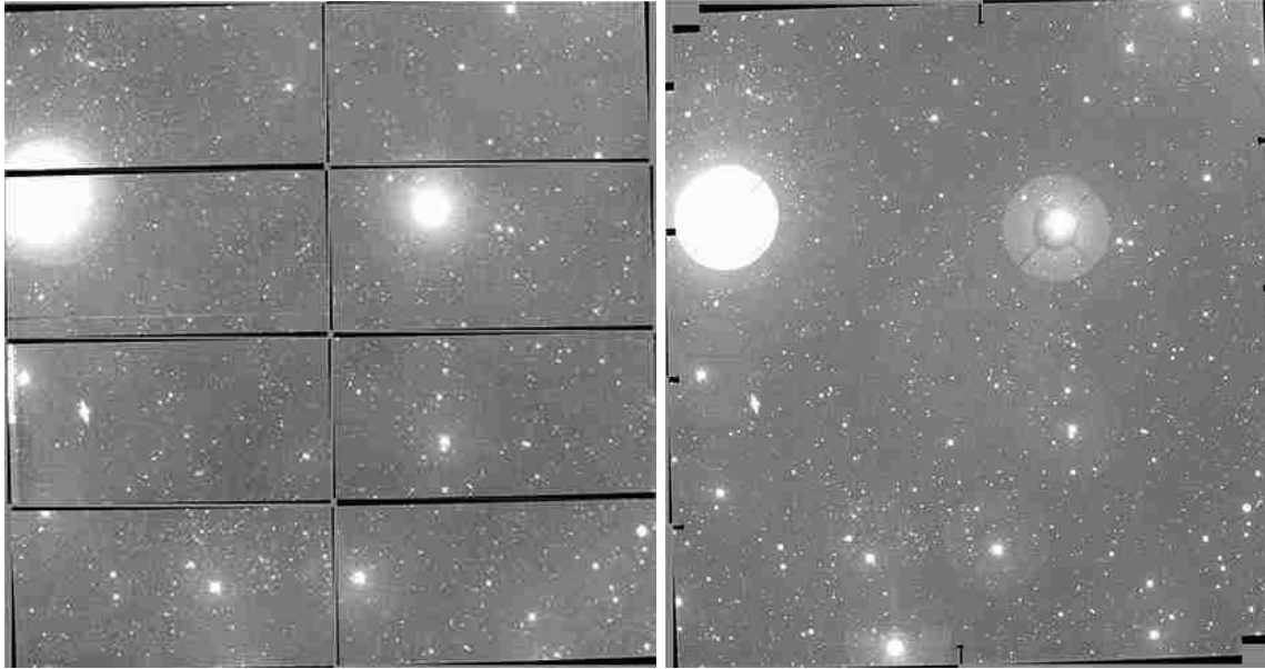
Figure 3.3 An image of field FN8-74, which has been processed using zero, dark, and flat images, but which has not been corrected by overlaying the dithered images to remove the missing regions between the 8 CCDs.
