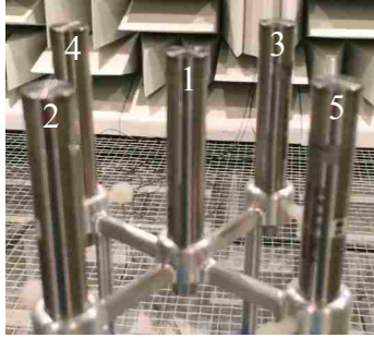
Figure 3.1: The multi-microphone probe used for the measurements in Chapters 3 and 4, labeled with microphone number labels. The rotation angle was 0^\circ when the speaker was on the same line as microphones 1, 2, and 3, and microphone 2 was the closest to the speaker.
