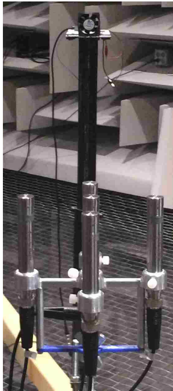
Figure 4.12: The setup for the fan noise experiment in an anechoic chamber. The fan is on the turntable and the probe is on a stand approximately 2 meters away.
