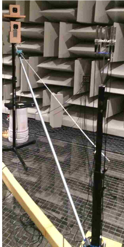
Figure 3.23: One variation of the two-speaker setup in an anechoic chamber. The speaker on the arm rotates, and the angle of rotation then becomes the same as the angle of separation between the speakers.
