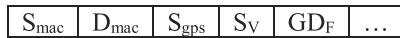
Fig. 4. An Illustration of a Broadcast Request Sent out from the Source Vehicle.
