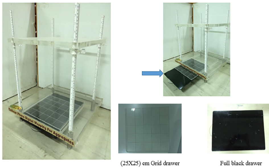
Fig. 7. Cellular phone digital mapping frame for coarse aggregate digital mapping mold for aggregate after implementation.
