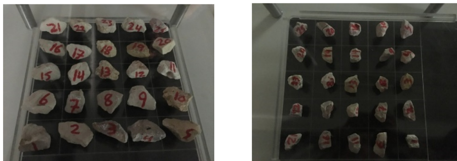
(a) large particles retained on sieve #1 (b) medium particles retained on sieve #1/2
