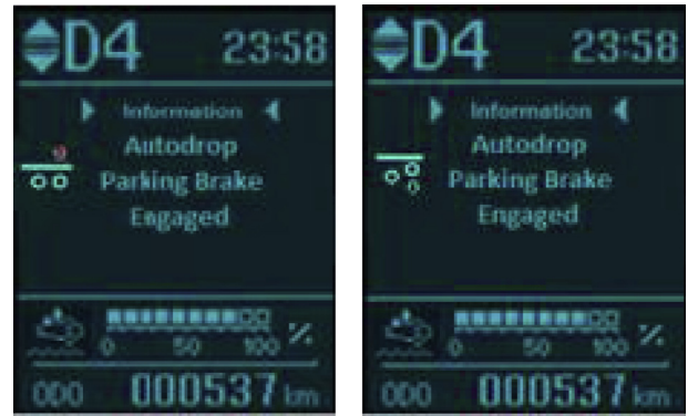
Fig. 15. Screen for the axle dropping system.
