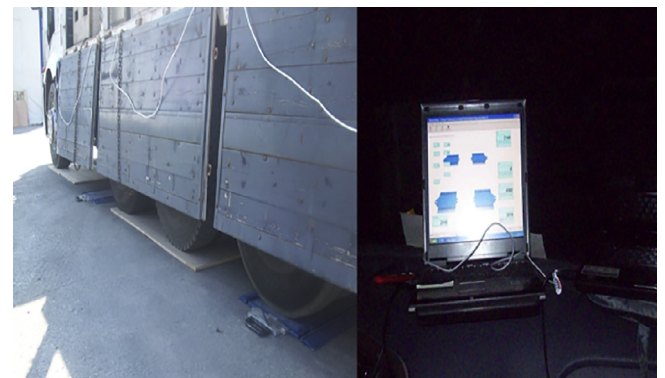
Fig. 7. Training Data Collection Tests (Axle Loads and Sensor output).
